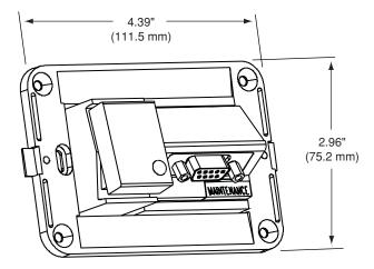
Figure 7: Switchplate Mounting Holes Layout
